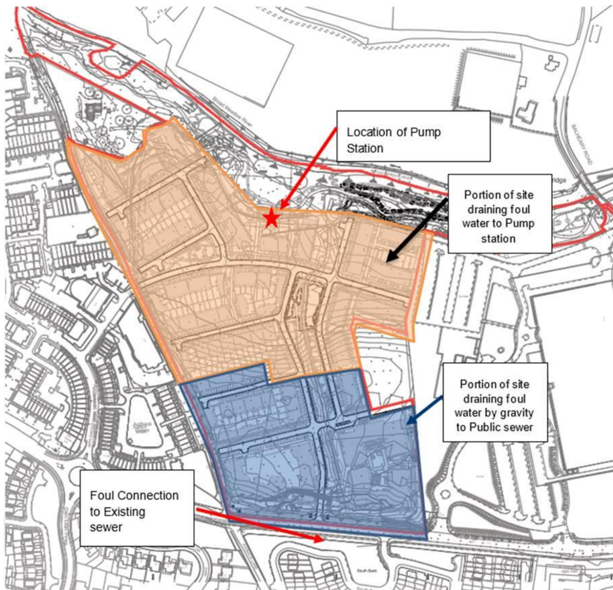
Figure 5-19 Location of pumping station (Source Engineering Assessment Report, WM)
